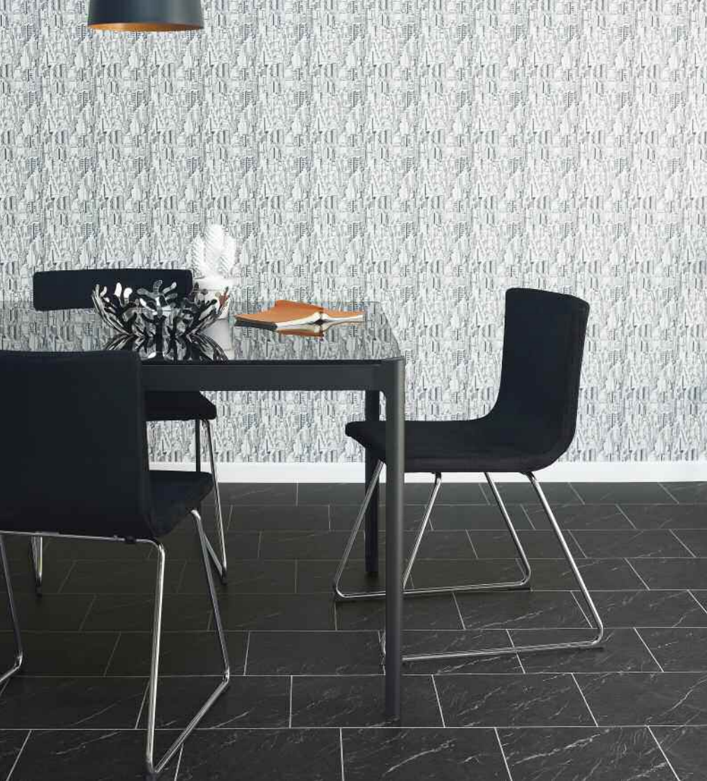
Installed with staggered joints with Grey Grouting Strip.
