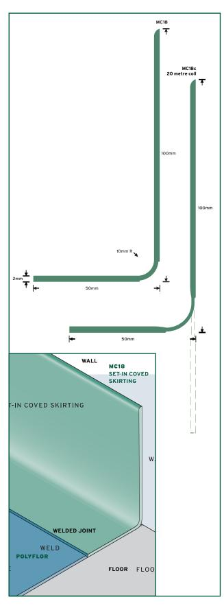
Skirting of this type is fitted before the flooring is laid, where a simple butt joint is required. Welded to the flooring, this provides a secure and impermeable joint. The benefits of a sealed, easily maintained surface are invaluable in hospitals and other similar locations where hygiene is of paramount importance.
