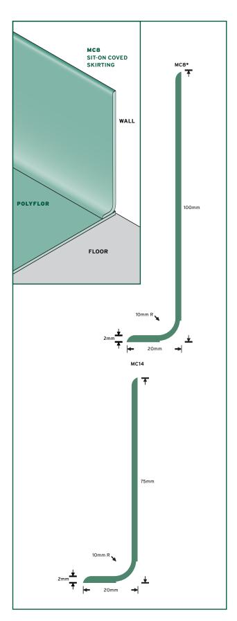
Sit-on coving is fitted after the flooring has been laid and can therefore be used to replace an old skirting, as well as to provide a neat finish to a new floor. These tough and durable covings give protection to the wall decorations at floor level. Ejecta skirting is easy to clean, needs no painting and offers long-term maintenance savings compared to timber skirting.
