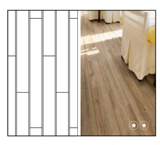
Straight laid plank with strip between each length ('ships decking' effect)
