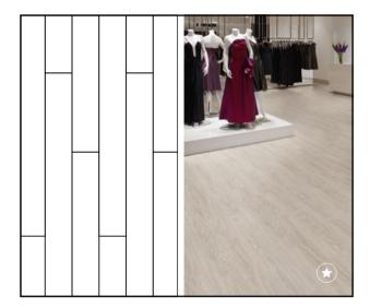
Straight laid plank - staggered
