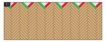
Continue this alternating installation of A and B planks throughout the remainder of the installation. It is important to check frequently that:
