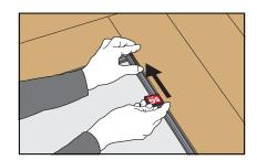
Align the 0.9mm wire with the installed 5G joint so that the wire is between the profile of the last installed plank and the flexible tongue. Push forward the 0.9mm wire into the joint. This pushes back the flexible tongue and releases the plank for dismantling.
